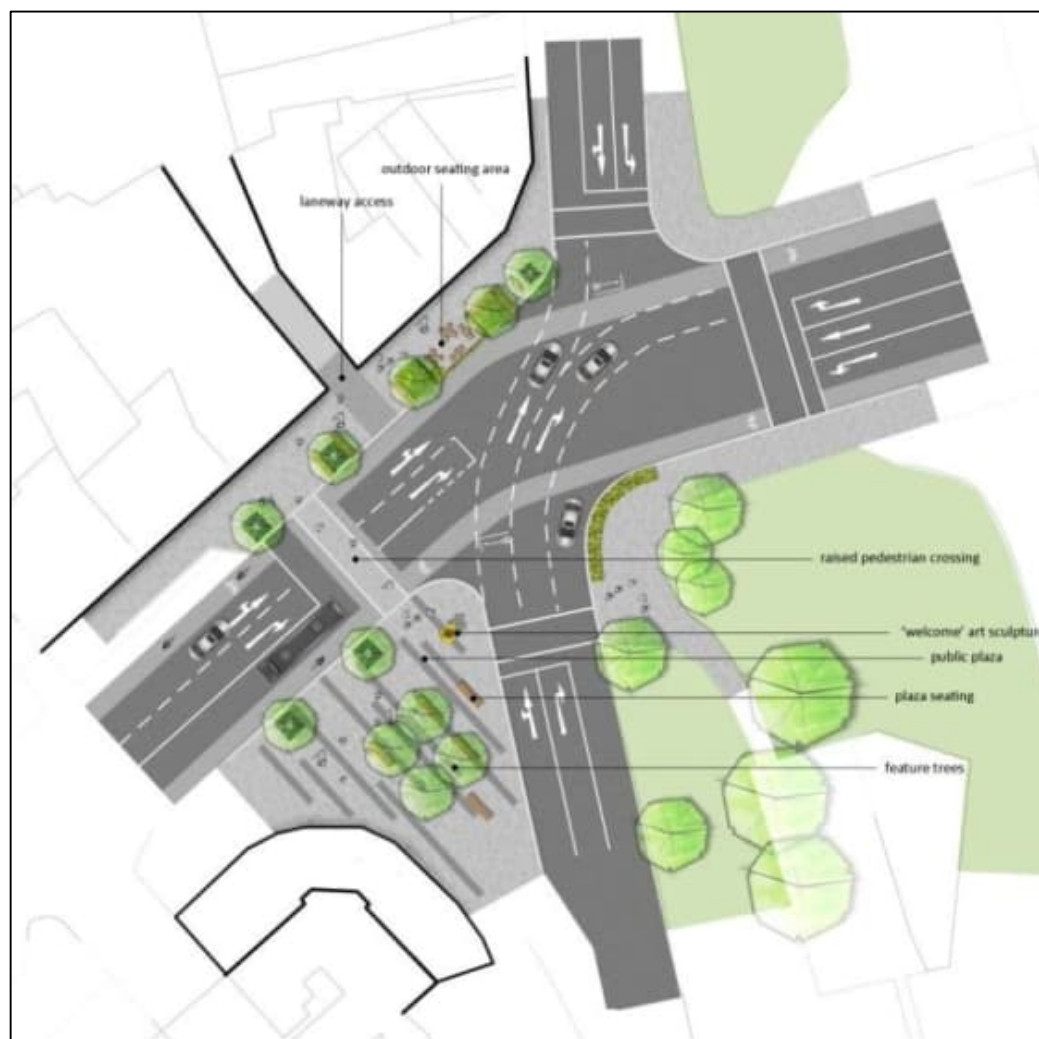
Figure 13. Conceptual NTA layout of the R445 Main Street and R416 Athgarvan Road Junction
